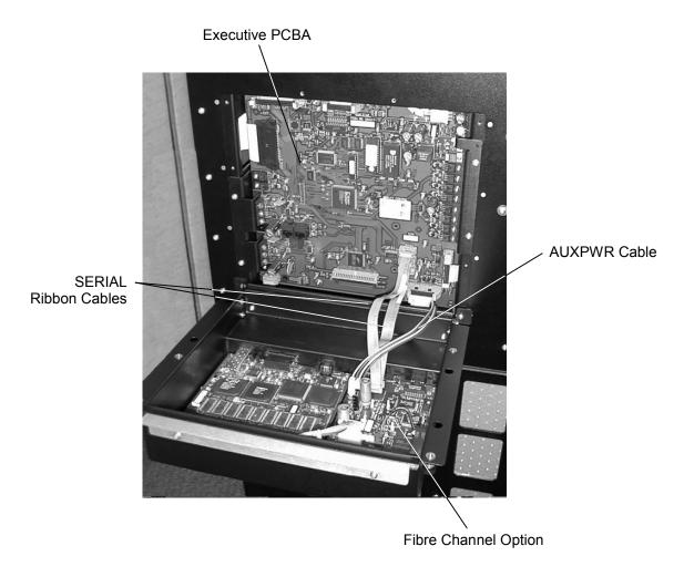
Figure 6-12 Executive PCBA and Fibre Channel Option (Executive IV PCBA Shown)
